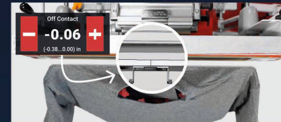
Digital off-contact adjustment right from the touchscreen control panel
