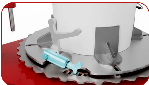
Adjust the clamp to your desired width and lock (step 1)
